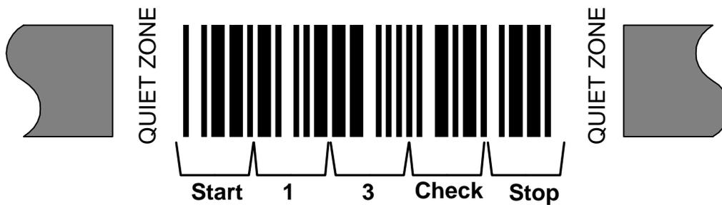
The basic structure of a bar code consists of a leading and trailing quiet zone, a start pattern, one or more data characters, optionally one or two check characters and a stop pattern.
