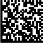
Data Matrix is a high density 2 dimensional matrix style bar code symbology that can encode up to 3116 characters from the entire 256 byte ASCII character set. The symbol is built on a square grid arranged with a finder pattern around the perimeter of the bar code symbol.
