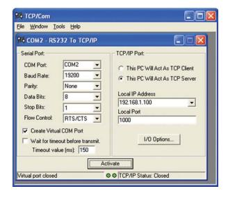
This would allow you to use WinWedge, TCP-Wedge, Telnet, HyperTerminal or any other RS232 or TCP/IP communications software to read or write to the serial device from any PC connected to the same network.
