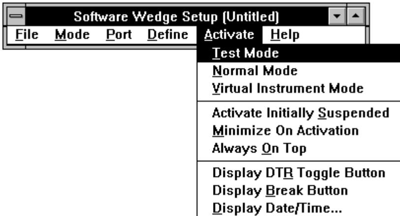
The "Activate" menu contains nine entries. The first three entries, "Test Mode", "Normal Mode" and "Virtual Instrument Mode" are used to activate the Wedge for serial input. The Wedge must be activated using one of these options before it will actually perform any serial I/O functions or transmit data to an application program. These three options and the differences between them are described in detail in the section: Activating The Software Wedge
