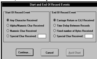
determine the start and end of each data record transmitted by our device. In this case each data record is a small text string ending with a carriage return (ASCII 13). Thus, we would specify “Any Character Received” as the “Start of Record Event” and “Carriage Return or CrLf Received” as the “End of Record Event”.
