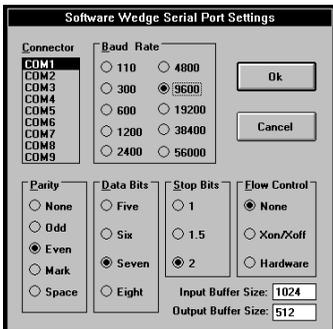
Step 2. Select the "SETTINGS" option from the "PORT" menu in the Software Wedge and choose the communications parameters COM1 (or COM2), 9600 baud, Even Parity, 7 Data Bits, two stop bits and no flow control from the dialog box that appears and then click the OK button to return to the main menu.
