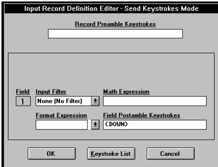
In the next dialog box to appear, place the cursor in the text box labeled “Field Postamble Keystrokes” and then click the button marked “Keystroke List”. When the keystroke list appears, scroll down through the list until the word “Down” is highlighted and then click the OK button in the keystroke list dialog box. This should cause the word “{DOWN}” to appear in the “Field Postamble Keystrokes” text box (as shown). Then click the button marked “OK” to return to the main menu.
