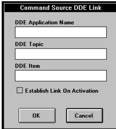
The dialog box is titled "Command Source DDE Link". It features three text input fields: "DDE Application Name", "DDE Topic", and "DDE Item". Below these fields is a checkbox labeled "Establish Link On Activation". At the bottom of the dialog are two buttons: "OK" and "Cancel".
