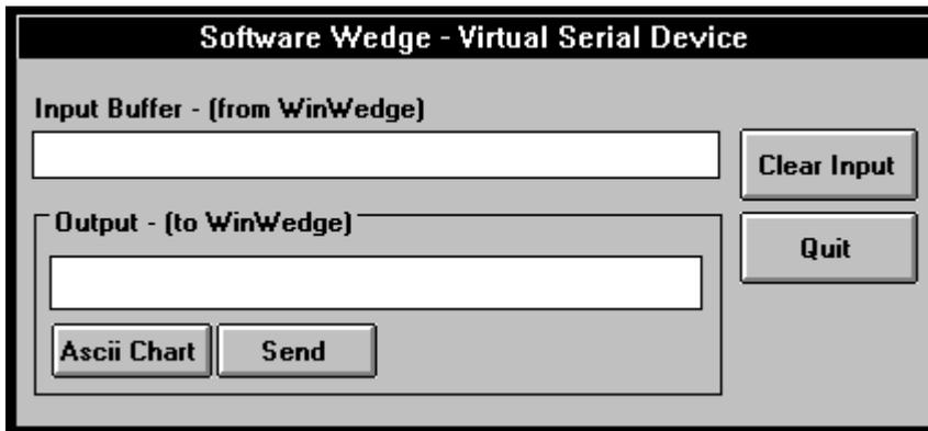
The virtual serial device dialog box allows you to test the functionality of the Wedge without requiring any real hardware device to be connected to a serial port on your PC. The dialog box has an “Input Buffer” that will display any data that would normally be transmitted by the Wedge out a serial port and it also provides an “Output Buffer” where you can enter and send data to the Wedge to simulate data that normally would be received from a device connected to an actual serial port.
