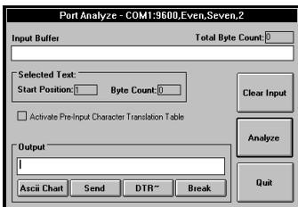
Step 3. Select "ANALYZE" from the "PORT" menu and transmit a sample reading from your device into the "Input Buffer" in the Analyze window. This step serves two purposes, first to simply test that your communications parameters are correct and that the device is connected properly and second to gain an understanding of how the data from the device is structured. If data does not appear in the text box marked "Input Buffer", then read the section of this manual entitled "Troubleshooting" .
