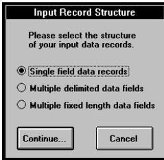
The next dialog box to appear provides options to describe an overall “Structure” for each data record. In this example our data only consists of a single “Field” therefore we would select “Single Field Data Records” and click the “Continue...” button.
