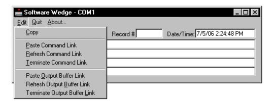
The *Copy* command allows you to copy the contents of one of your input data fields, the record number or the date/time display into the Windows clipboard. To use this feature, click your mouse in the text box that you want to copy and select "Copy" from the menu. Any data copied from WinWedge can be either *Pasted* or *Paste Linked* to other Windows applications.
