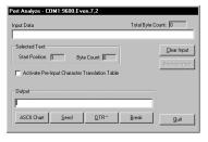
Step 3. Select "ANALYZE" from the "PORT" menu and transmit a sample reading from your device into the "Input Buffer" in the Analyze window. This step serves two purposes, first to test that your communications parameters are correct and that the device is connected properly and second to gain an understanding of how the data from the device is structured. If data does not appear in the text box marked "Input Buffer", then read the section of this manual entitled "Troubleshooting" (pg. 104).
