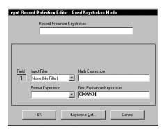
In the next window to appear, place the cursor in the text box labeled "Field Postamble Keystrokes" and then click the button marked "Keystroke List". When the keystroke list window appears, scroll down through the list until the word "Down" is highlighted and then click the OK button in the keystroke list window. This should cause the word "{DOWN}" to appear in the "Field Postamble Keystrokes" text box (as shown). Then click the button marked "OK" to return to the main menu.
