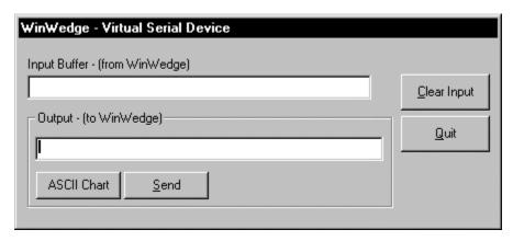
The virtual serial device window allows you to test the functionality of WinWedge without requiring any real hardware device to be connected to a serial port on your PC. The window has an "Input Buffer" that will display any data that would normally be transmitted by WinWedge out a serial port and it also provides an "Output" textbox where you can enter and send data to WinWedge to simulate data that normally would be received from a device connected to an actual serial port.
