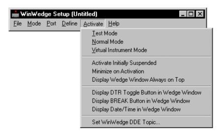
The "Activate" menu contains nine entries. The first three entries, "Test Mode", "Normal Mode" and "Virtual Instrument Mode" are used to activate WinWedge for serial input. WinWedge must be activated using one of these options before it will actually perform any serial I/O functions or transmit data to an application program. These three options and the differences between them are described in detail in the section: Activating WinWedge (pg. 51)
