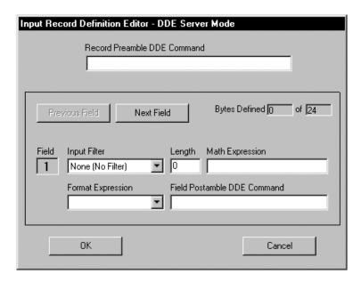
All of the controls in the above window are the same as when WinWedge is in "Send Keystrokes Mode" except that instead of supporting *Record Preamble Keystrokes* and *Field Postamble Keystrokes*, the window allows you to enter a *Record Preamble DDE Command* and *Field Postamble DDE Commands*. Most applications that support DDE also support a set of *DDE commands* that may be issued to them by other application programs (such as WinWedge).
