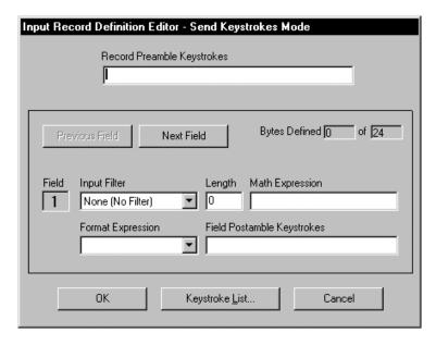
The lower half of the window is where you specify an "Input Filter" to be applied to each data field in your input records as well as an optional "Math Expression", an optional "Format Expression" and a "Field Postamble". In cases where each data field consists of a fixed number of bytes, you must also specify a field "Length".
