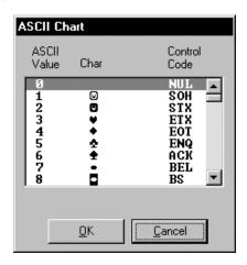
Note: When using WinWedge in DDE Server Mode, characters translated to "Nul" in the Pre-Transfer Character Translation Table will be removed from the outputted data. Translating characters to NUL can thus be used to remove unwanted characters. In Log To Disk Mode, all Nul characters (ASCII 0) and characters translated to "Nul" are written to disk along with the rest of your data.
