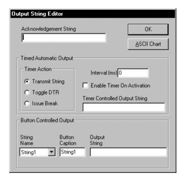
The Acknowledgment String is a character string that is automatically sent out the serial port after each complete data record is received from your serial device. The capability to send an Acknowledgment string was originally intended for those devices that require an acknowledgment (an ACK character for example) but it could also be used as a way to continually request data from a device that can be polled by sending it a character string.
